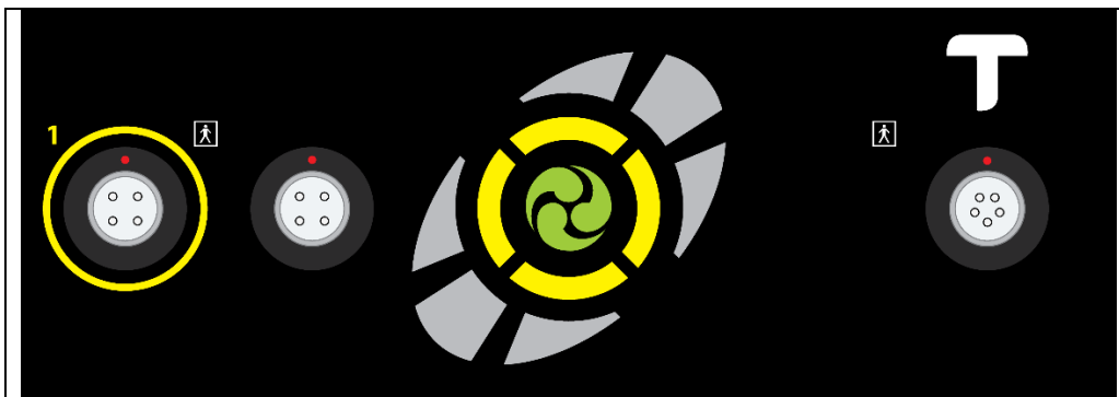
Figure 12: Channel 1, Cement Transducer Active
